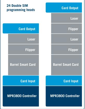
All configurations are available with an optional additional input and output module and/or an additional smart card module.
